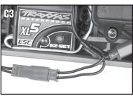
Plug the red male connector from the power Y-harness into the red female connector from the tail lights harness.
